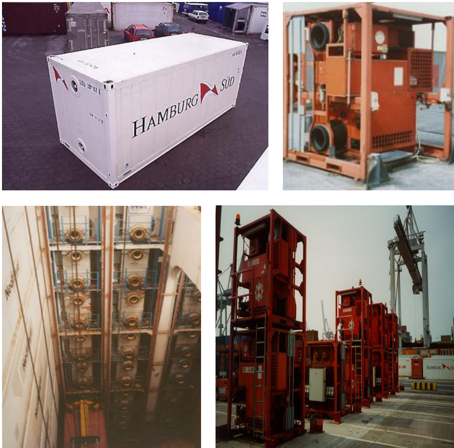
Figure 2. The porthole container system: a) porthole container, b) clip-on unit, c) the hold of a container ship adapted to carry porthole containers, d) terminal-based refrigerating system
