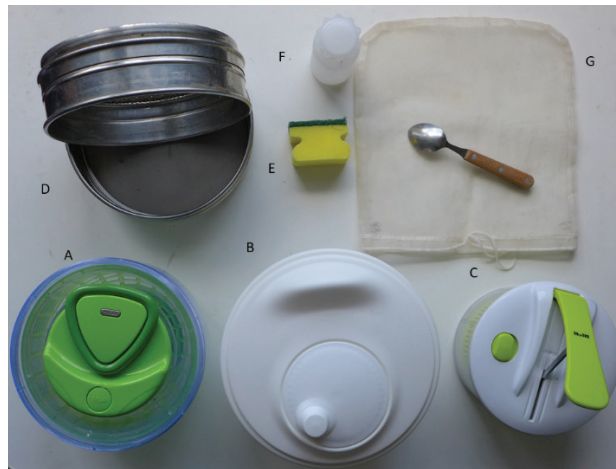
A – pull-cord spinner; B – crank-operated spinner; C – push-bottom spinner; D – two metal sieves with a mesh size of 3.2 mm and 0.250 mm, respectively; E – sponge; F – 125-ml plastic jar; G – 0.200 mm nylon mesh bag and spoon.
